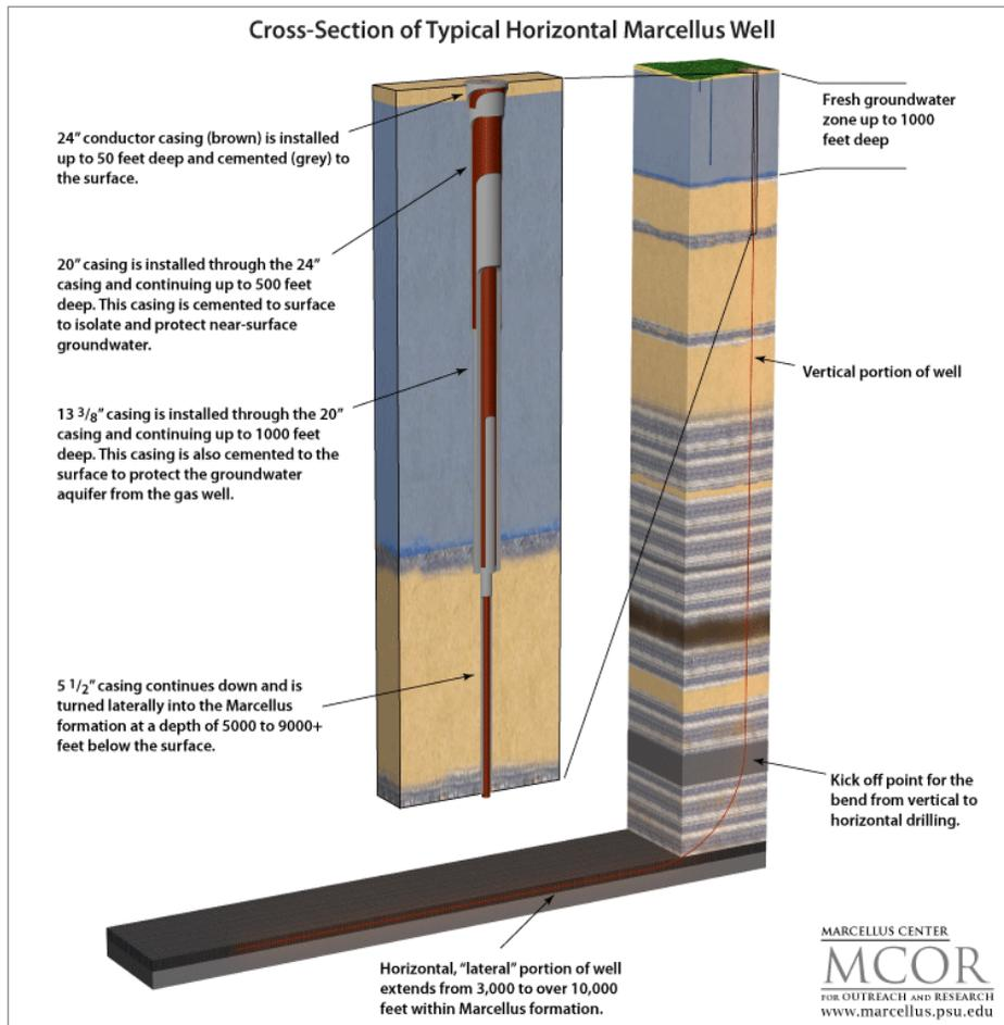
When drilling an unconventional well, operators begin by drilling a vertical wellbore from 5,000 to 9,000 feet into the shale rock. As the vertical wellbore is drilled, various diameters of steel pipe called "casing" are cemented into place in the wellbore. This casing protects groundwater aquifers from pollutants inside the well and helps to stabilize the wellbore as the operator drills farther into the subsurface. The casing also keeps surface water and other geological
